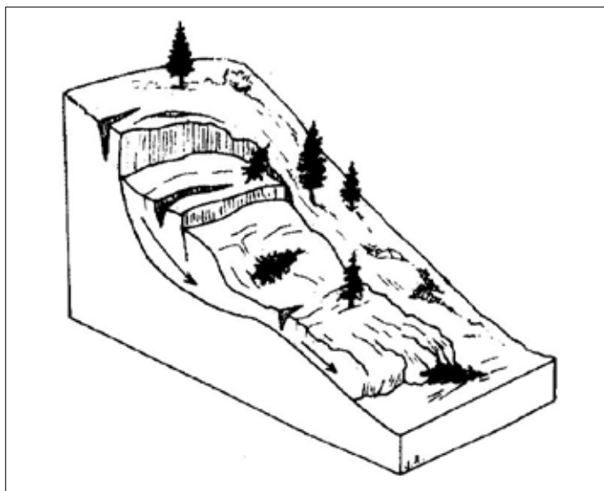
Figure 1. Diagrammatic sketch of a translational/rotational landslide. Drawing by Janet Appleby Richard Killbourne and Thomas Spittler; modified from Varnes (1978)
